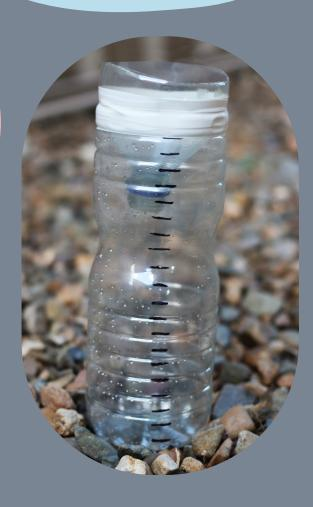
5. Set the rain gauge in position and make sure it is level. If needed, you can dig a small hole in the ground to hold the bottle securely.
